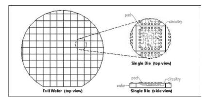
Figure 1-1: Integrated Circuit Wafer
